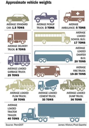
**Figure 1**: Typical weights of various vehicles. Although overall vehicle weight has an impact on roadways, the distribution of the weight over the axles of the vehicles has a greater affect. *Source*: Pennsylvania Department of Transportation.
