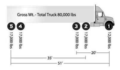
**Figure 2**: The weight of a fully loaded tractor trailer and its distribution over its axles. The axle weights for trucks hauling sand is heavier than semis because they have fewer axles and as a result, their per-axle weight and their subsequent impact on roads will be greater. *Source*: Utah Department of Transportation, "Chapter 21, Bridge Table Calculations," July 5, 2013, http://www.udot.utah.gov/main/f?p=100:80:0:::1:T,V:4206.
