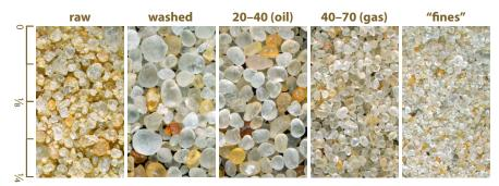
▲ Frac sand as it appears at the quarry (raw), washed to remove clay minerals, and sorted by size for various uses (number ranges identify openings per inch in the sorting sieves). Sand that is too small for use in hydraulic fracturing ("fines") may be used as fill for mine reclamation, as cow bedding, or for other purposes.
